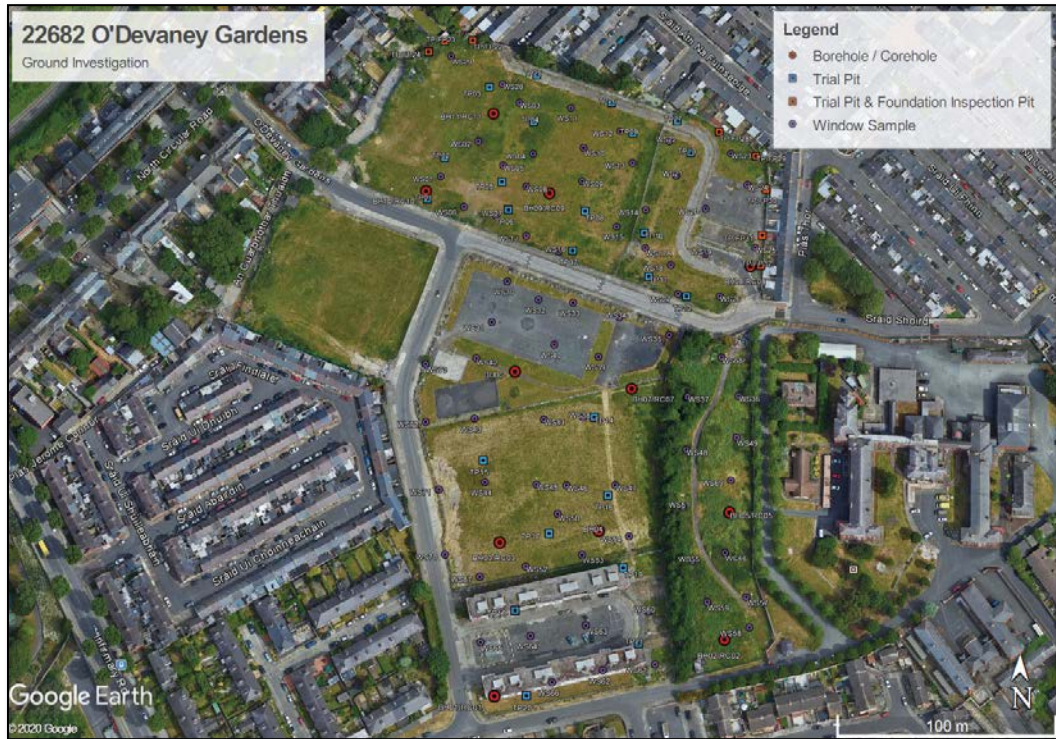
Figure 7 – Extract from IGSL Site Investigation indicating sampling locations
